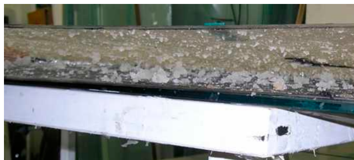
Figure 6. Soft siloxane clusters can be easily collected and recycled into silicone rubber.
