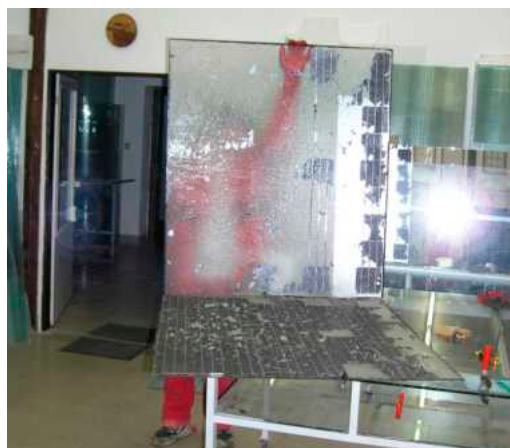
Figure 5. Separation of nondamaged glass sheets with the remaining siloxane gel.
