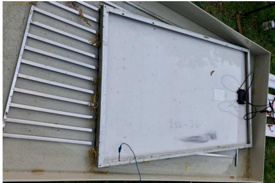
Figure 2. Photograph of the actual laboratory installation with the PP tank, immersed module and insulation tester.
