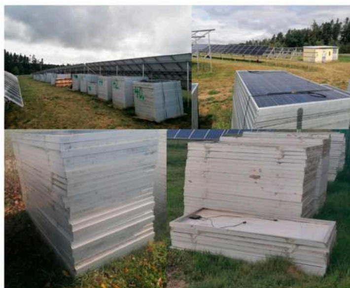
Figure 1. Anonymized field photographs showing damaged PV modules stored directly on grass/soil within fenced PV parcels.
